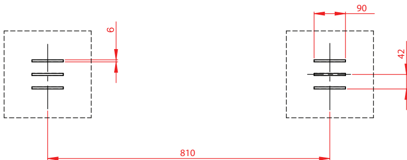
EMBEDDED ELEMENTS SPACING (SCALE 1:10)
