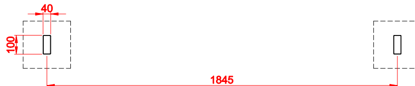
MOUNTING HOLES SPACING
